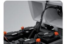
The detergent water tank serves as battery compartment, allowing the housing of great capacity batteries granting continuous working time up. Large capacity shock and acid proof polyethylene tank (1101) improves productivity avoiding frequent refilling and idle time.
